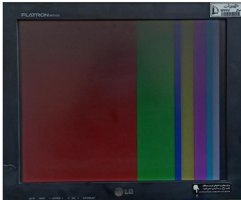
Fig. 4. Real-time display of the CNN model's probability map on the CIFAR-10 dataset during the testing phase. The width of each color bar indicates the predicted probability of the corresponding class, with the widest bar representing the most likely classification.
