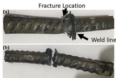
Figure 1. Fracture surfaces of the rebars: (a) in the base metal, (b) in the weld
