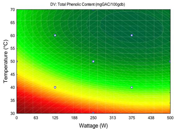
Fig. 7. (a) Response surface and (b) contour of the total phenolic content (mg GAC/100 g<sub>db</sub>) of red seaweed (*Chondracanthus chamissoi*) dried with hot air assisted by incandescent lamps
