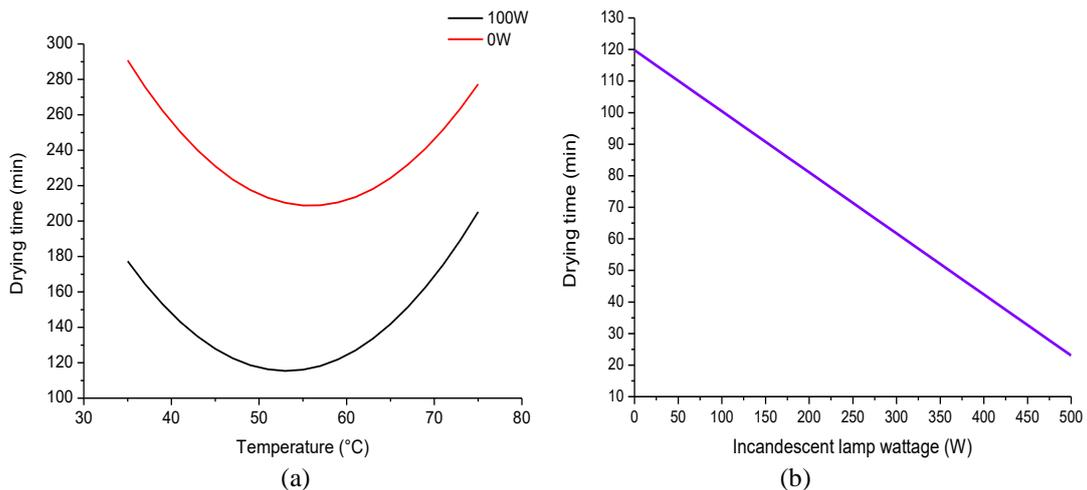
**Fig. 12.** (a) Behavior of the drying times versus air temperature for two values of the incandescent lamp wattage with constant drying air velocity (1.5 m s<sup>-1</sup>) and charge density (4.0 kg m<sup>-2</sup>); (b) Graphical simulation of the drying times of the red seaweed for variations of the incandescent lamp wattage
