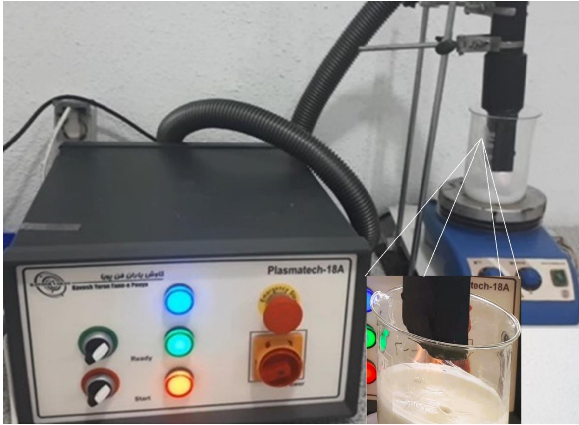
Fig. 1. The experimental setup for the cold plasma irradiation of starch/ZnO NPs film-forming solutions using a jet cold plasma system
