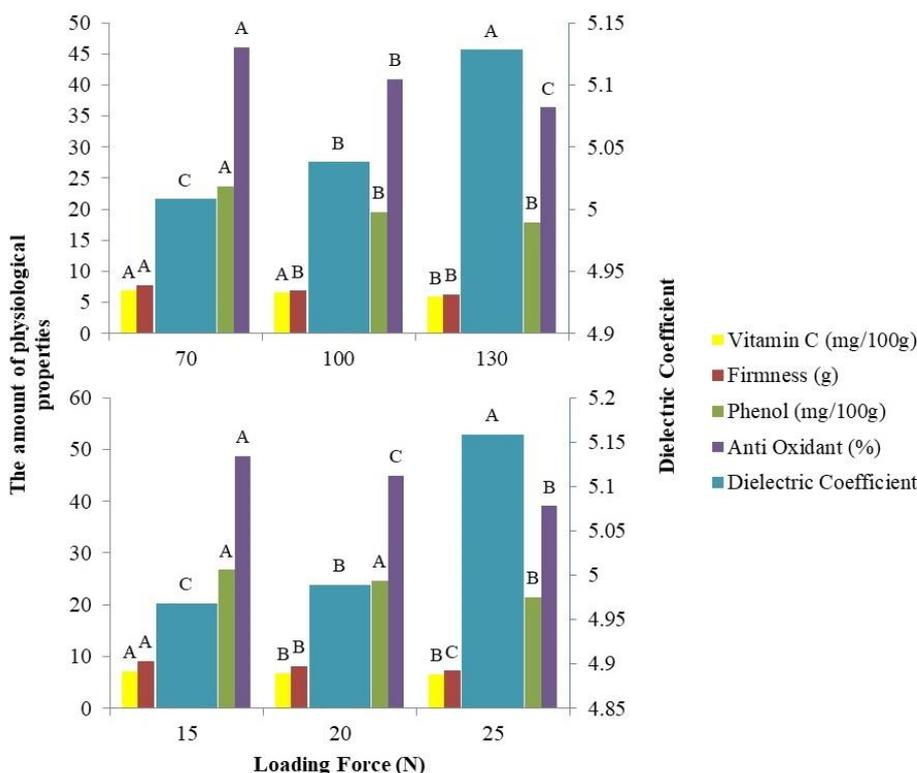
**Fig.4.** The effect of loading forces on the qualitative properties and the dielectric coefficient in wide-edge compression and thin-edge compression. Similar letters of every property indicate the absence of significant difference.
